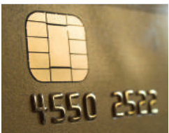
Figure 2.3 The chip on a smart card
